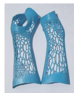
Figure 4d: The two halves of the 3D printed orthopedic forearm cast
