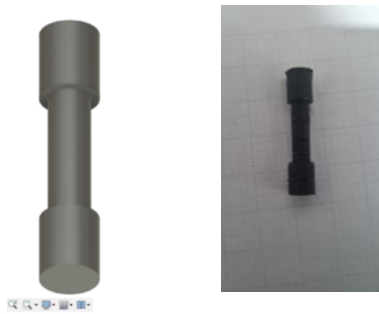
Figure 5: Sample designed in fusion 360 and 3D printed sample
