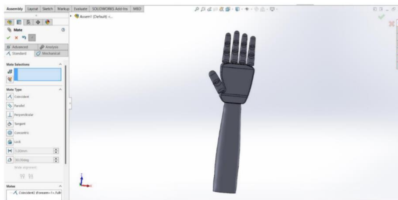
Figure 2: Fully assembled hand and forearm model in SolidWorks showing aligned finger joints, palm structure, and forearm connection.
