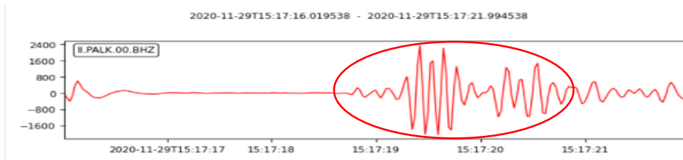
Figure 2: Identify the P and P code wave from the continuous seismic wave. Here, both P and S wave were selected because the event was small therefore this could be the time window.
