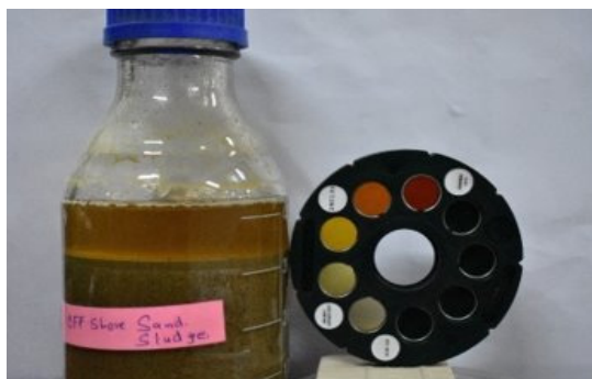
Figure 02: Reagent bottle supernatant liquid color is darker than the standard color
