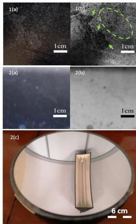
**Figure 1:** 1(a) and 1(b) indicate contamination of the thin films due to residuals of the cleaning agents (arrows) and pin-holes formed due to water vapour adhered in the glass (inside the circle). 2(a) and 2(b) illustrate a coat with minimum contaminants which was coated in a greater vacuum whilst image 2(c) contains the full view of the coated, f/2 254 mm diameter telescope primary.
