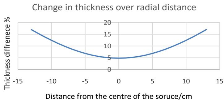
**Figure 2:** The uniformity change with the radial distance from the centre of the source. Generally, a SiO protective coating is applied on telescope primaries and it will protect the Al coating from rapid degradation. However, this protective coating may introduce new errors to the coating [4] and require further modification in the modified thermal evaporator. Therefore, the effect of the protective coating is not discussed here.
