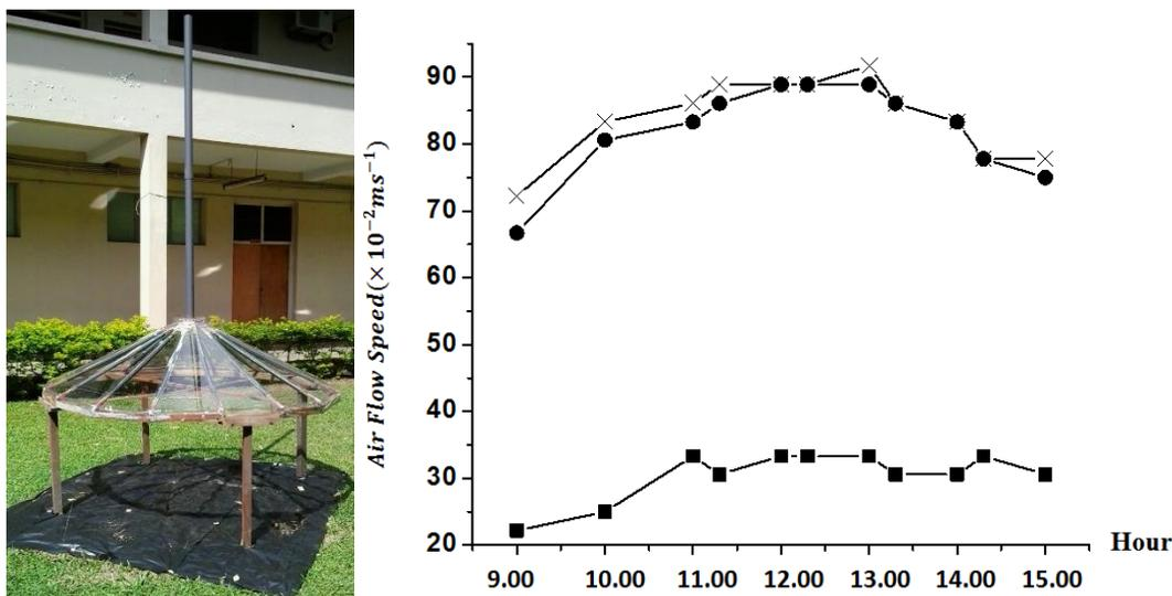
Figure 4: (a) The model chimney dryer in open air (b) Variation of air flow speed (under the collector: x- Natural flow with grass O- covered by black polythene (■) Variation of the environmental wind speed.
