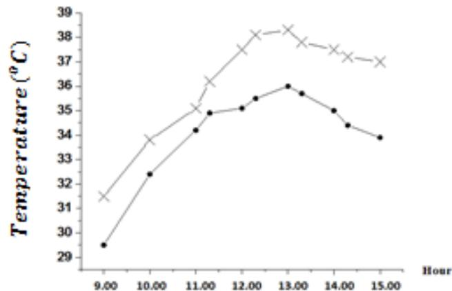
Figure 5: (a) Variation of the inside temperature of the chimney (×) and the environmental temperature (•) during 9.00 -15.00.
