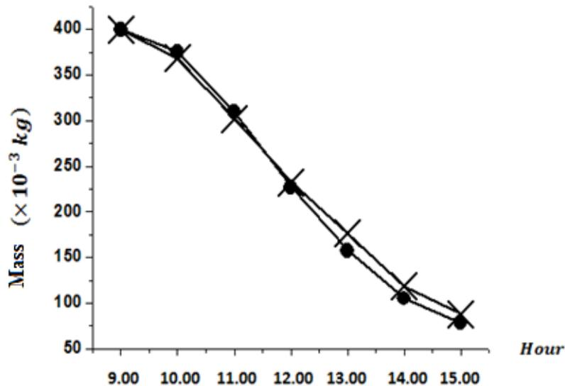
Figure 6: Mass of the refuse coir under solar drying and sun drying ((●) - sun drying (×) - Solar drying)
