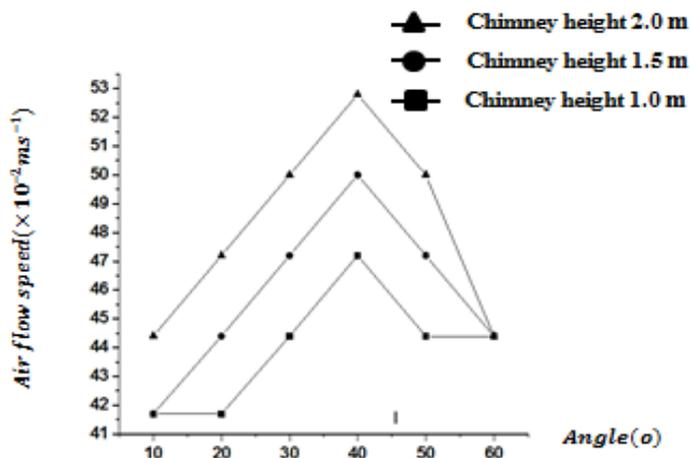
Figure 3: Variation of the air flow speed with the collector angle (lines have been drawn to guide the eye)
