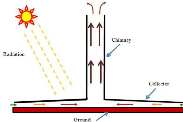
Figure 1: Sketch of a Solar Chimney
