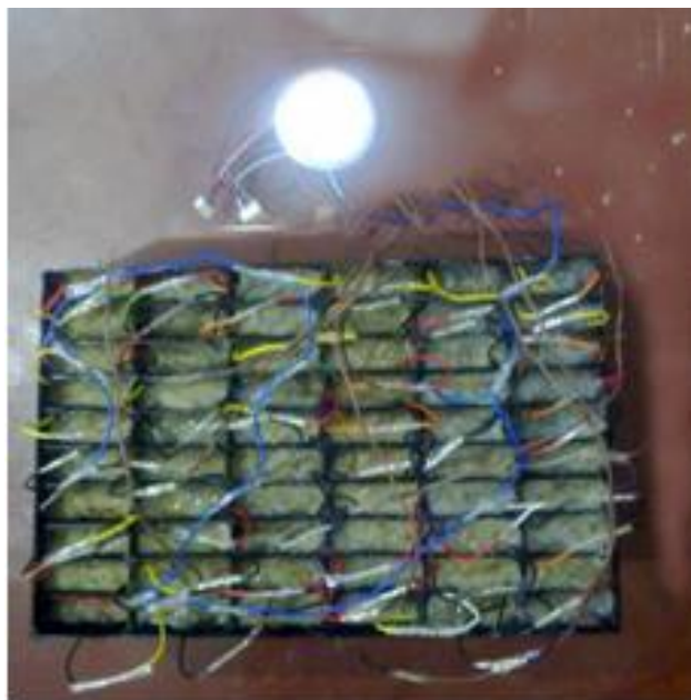
Fig. 3: Plantain pith battery powered 3 W lighting system
