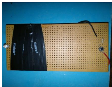
Figure 2: Device with an IR LED and Push-button
