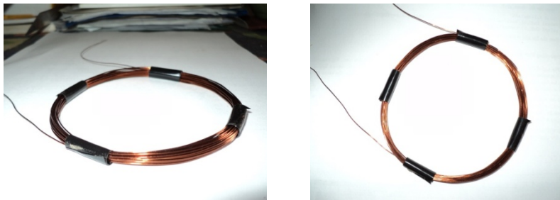
Figure 2: A constructed inductor coil for the purpose of metal detection
