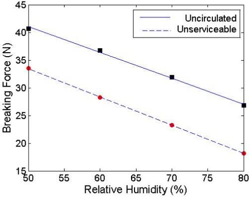
Figure 4 : Variation of breaking force with relative humidity
