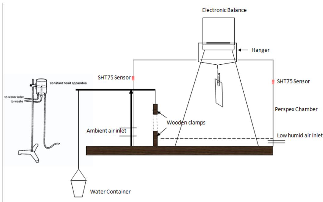
Figure 1 : Schematic diagram of humidity control chamber
