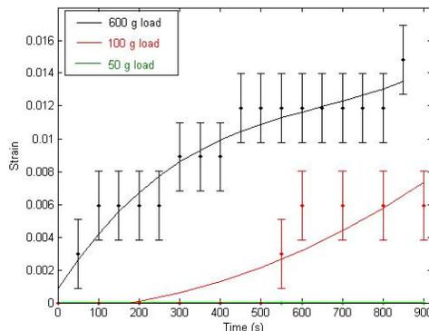
Figure 7 : Creep curves for uncirculated notes under different applied forces
