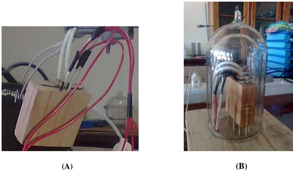
**Fig 1 (A) A plane heater inserted into a wood sample of cuboid shape. The sensing elements of thermistors are inside the wooden block (B) Wood sample mounted on base and covered by vacuumed glass chamber to minimize radiation heat loss**
