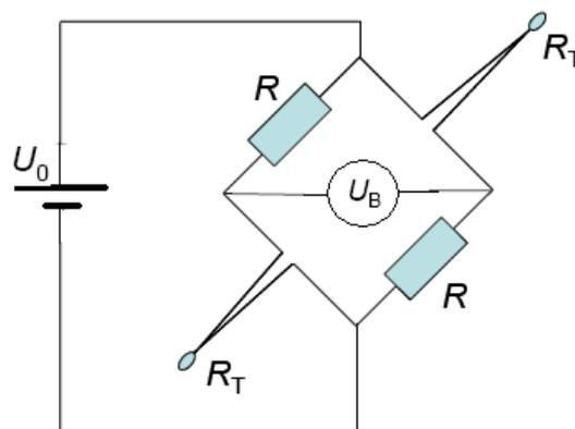
**Fig. 2 Schematic diagram of Wheatstone bridge circuit to measure thermal capacity of wood**
