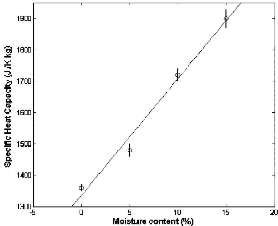
**Fig. 5: Relationship between Specific heat capacity and moisture content**
