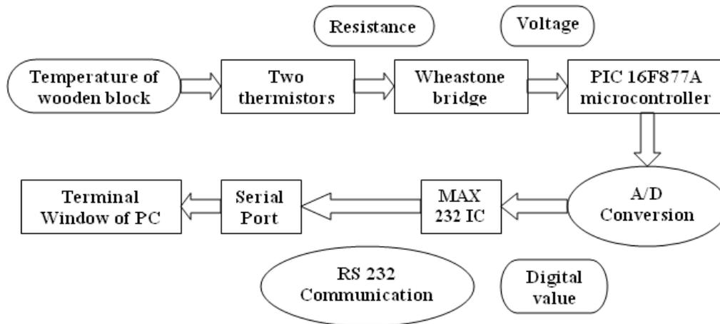
**Fig 3 Block diagram illustrating of temperature measurement using Wheatstone bridge method**
