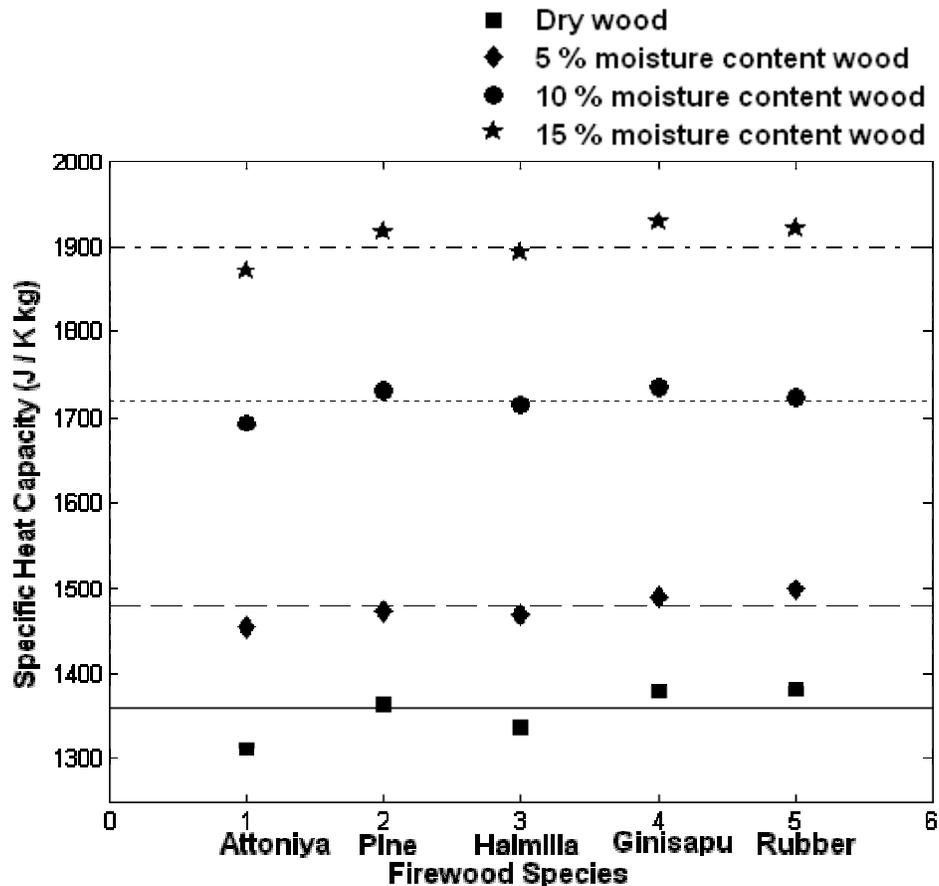
**Fig. 4 Variation of specific heat capacity of wood species for dry wood and for wood with different moisture content levels**
