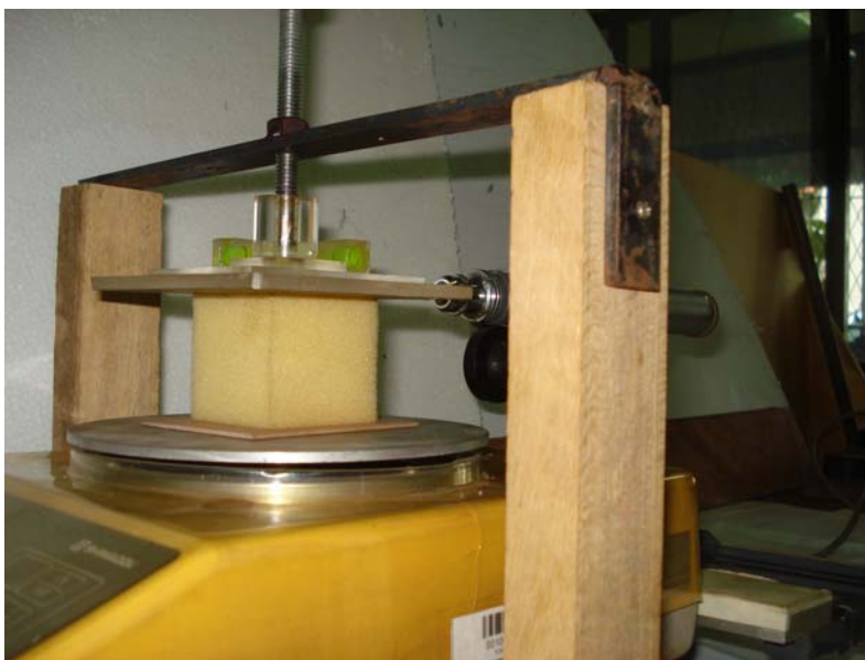
Fig. 1: The experimental setup used to measure linear stress-strain behaviour of foam materials
