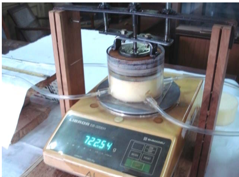
Fig. 2: The experimental setup used to measure volumetric stress-strain behaviour of foam materials
