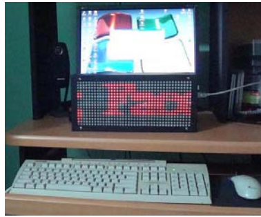
Figure 3: The microcontroller controlled LED display panel of the system
