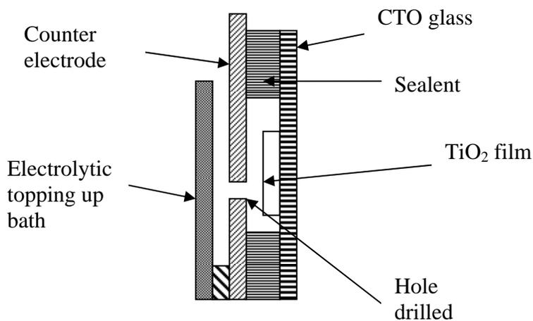
**Figure 2: PEC cell with electrolytic topping up bath**
