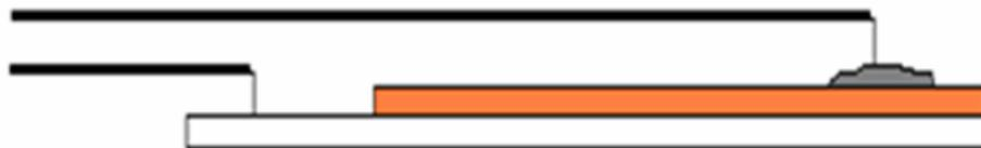
Figure 2- Electric connections on the thin film, first method
