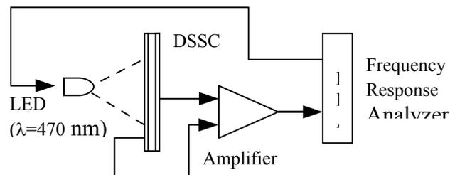
**Fig 3** Schematic diagram of experimental set up for IMVS and IMPS measurements
