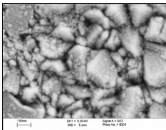
**Fig.1** SEM picture of gold nano particle embedded SnO<sub>2</sub> film
