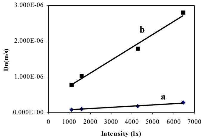
**Fig. 5** Diffusion coefficient of dye-sensitized solar cells of (a) SnO<sub>2</sub> and (b) Au/SnO<sub>2</sub> films at different light intensities ( $\lambda = 470$  nm)
