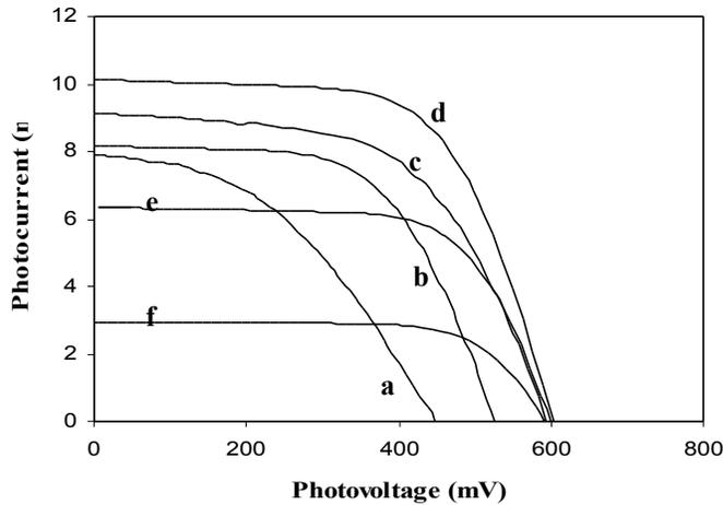
**Fig. 2** I-V characteristic curves of dye-sensitized solar cells of Au/SnO<sub>2</sub> composite films made of (a) 0 % (b) 4.7x10<sup>-4</sup> (c) 9.4x10<sup>-4</sup> (d) 1.41x10<sup>-3</sup> (e) 1.88x10<sup>-3</sup> (f) 2.35x10<sup>-3</sup> of gold by weight.
