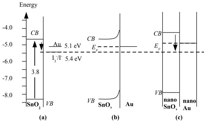
**Fig. 6** Band diagram of (a) SnO<sub>2</sub> (b) SnO<sub>2</sub> and gold Schottky junction (c) SnO<sub>2</sub> and gold nano-particle contact.
