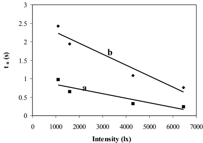
**Fig. 4** Lifetime of germinated electrons in dye-sensitized solar cells of (a) SnO<sub>2</sub> and (b) Au/SnO<sub>2</sub> films at different light intensities ( $\lambda = 470$  nm).
