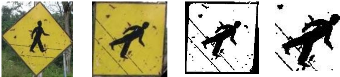
Figure 5: (a) Identified road sign region (b) Extracted region after Radon transformation (c) Binarized image (d) Cropped image (96x96)
