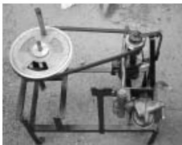
Figure 3: Manually Designed Oil Filter System
