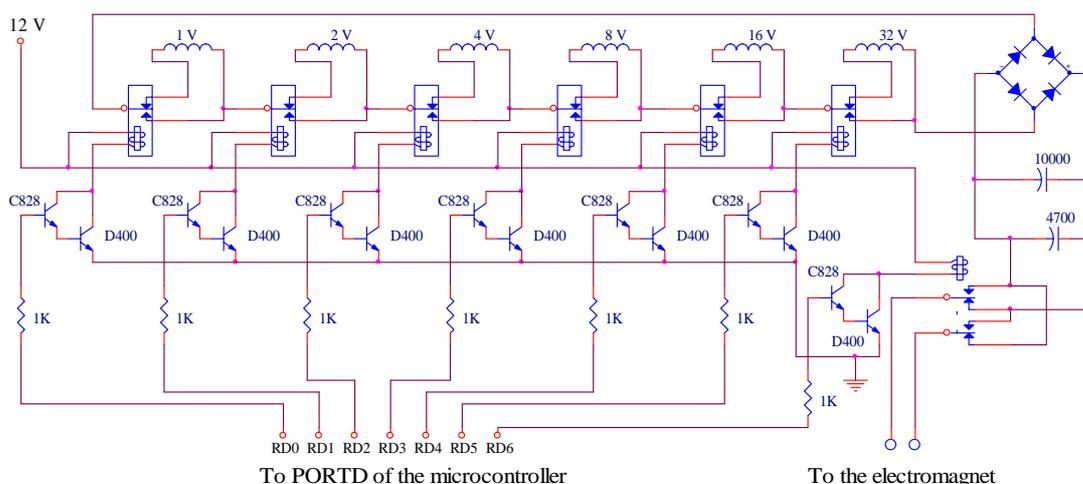
Figure 2.2: Voltage controller circuit
