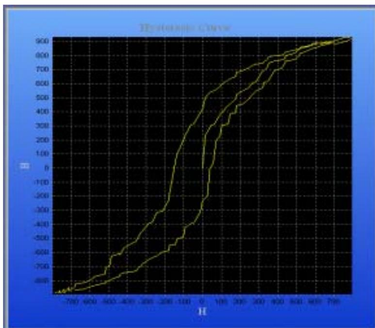
Figure 4.1: Hysteresis loop obtained for an Iron sample
